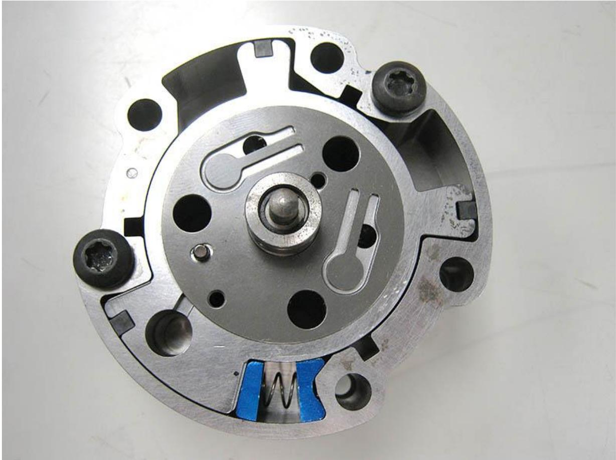
6. The torque for the bolts is 135 in lbs. We recommend using a small dab of blue thread locker on each bolt.
