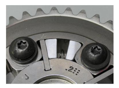
7. The torque for the bolts is 145 in lbs. We recommend using a small dab of blue thread locker on each bolt.
