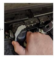
(2) Connect supplied MGD1 adapter cable to the "VEH" connector, and securely lock it in place. This is typically the connector closest to the outside of the truck, but please verify before connecting.
