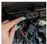
v) Connect MyCalibrator tuner to adapter cable
