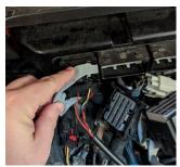
(3) Connect MyCalibrator tuner to adapter cable
