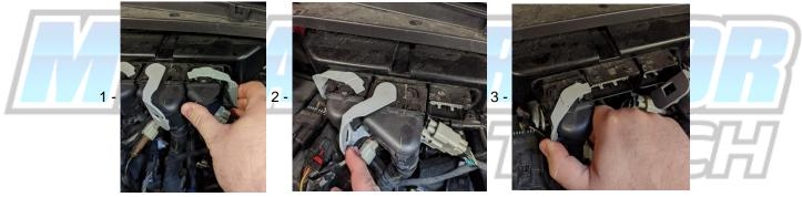
v) Connect supplied LME adapter cable to the "VEH" connector, and securely lock it in place. This is typically the connector closest to the outside of the truck, but please verify before connecting.
