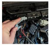
(3) Connect MyCalibrator tuner to adapter cable
