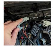
vi) Connect MyCalibrator tuner to adapter cable
