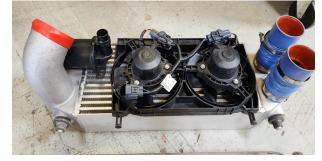
17. (Raptor Only) Install the fans onto the intercooler and factory support bracket prior to reinstall, these will no longer have any grommets installed, it is by design to have the plastic in direct contact with the support bracket.
