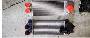
14. Mount the bypass valve to the new intercooler with the supplied 6mm socket head cap screw bolt. Torque to 55 in-lbs.
