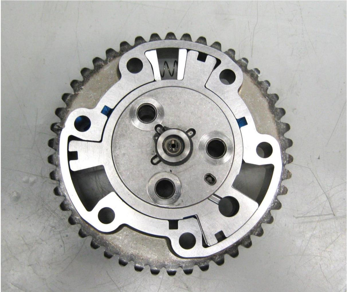
6. The torque for the bolts is 135 in lbs. We recommend using a small dab of blue thread locker on each bolt.
