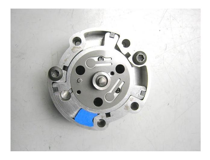
6. The torque for the bolts is 135 in lbs. We recommend using a small dab of blue thread locker on each bolt.
