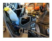
7. Remove plastic bracket under the air-box by pulling straight up. Note: use care when removing as there is a wire that must be removed from the bottom corner.
