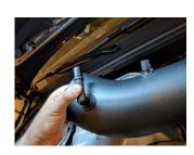
11. Reinstall the factory PCV vacuum fitting on new intake tube. (2019+ models differ)
