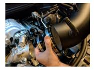
**13.** Fit the 4"-5" coupler onto the new air-intake tube along with one 4.25" and one 5.25" hose clamp.
