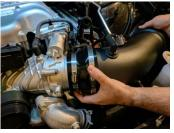
**14.** Slide silicone coupler with hose clamps onto the throttle body.
