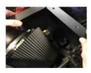
17. Install the new air-box by carefully pushing down directly onto mounting tab till locks in place. Do NOT push down on top of the box as tabs bend easily.
