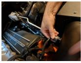
**21.** Reconnect the inlet air temp sensor connection.
