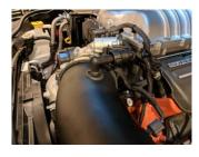
22. Reinstall the factory PCV hose. (2018 only, 2019+ see step 18 and utilize supplied fitting and hoses)
