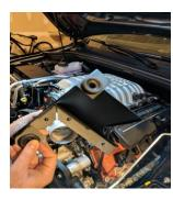
**12.** Reinstall the factory grommets onto the new airbox. Refer back to step six.
