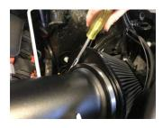
**16.** Install supplied air filter. Ensure that hose clamp is secure and tight. Note: Filter should be parallel with air-box lid
