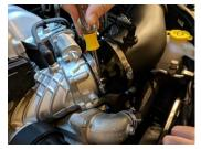
**15.** Tighten the 4.25" hose clamp at the throttle body.
